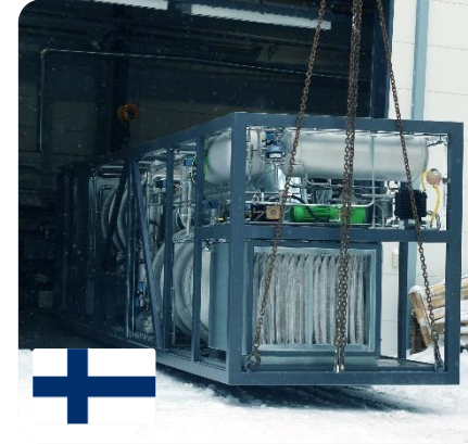
HVAC integrated CO 2 capture unit in a factory in Vantaa, Finland
